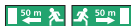
L19 Nearest exit or second nearest exits in the directions and at the distances indicated on the sign
