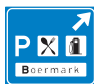
K3 Information sign for exit to motorway service area, showing the name of the rest area and symbols for the services offered
