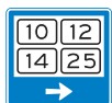
K13 Signpost within a built-up area showing district numbers (in traffic areas)
