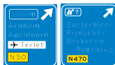
K2 Advance warning sign for an exit on a motorway showing the distance to the exit, the exit number, destinations after the exit (top destination is the name of the exit), direction to aerodrome/airport and the non-motorway road number
